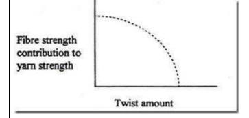
On the other hand, as yarn twist is increased, the frictional resistance between the fibres gradually increases until a point is reached at which slippage is virtually impossible. The relationship is illustrated in the diagram below:
