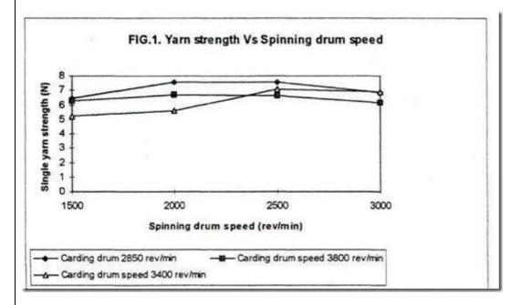
The strength of the yams depends on two principles factors - the fibre strength and the frictional resistance to slippage2.
