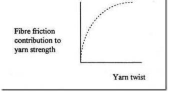
The effect of twist/spinning drum speed on the strength of dref yarns is, therefore, determined by a combination of the two effects just described above, and the resulting relationship is as illustrated in Figure 1.
