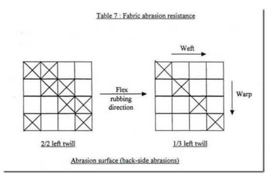
When we examine the two structures to be abraded, it is noticed that there is more west-floating on the back of 3/1 twill than the 2/2 twill. This results in a higher degree of exposure of west yarns to be abraded and a lower abrasion resistance which appears on the back of 3/1 twill fabric.
