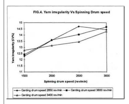
From Figure 4, it is found that when the spinning drum speed increases, the yarn irregularity (CV%) increases. Besides, the Figure shows that carding drum speed contributes little influence on the CV% value. As the spinning drum speed/twist increases, the mean yarn volume decreases, making the yarn more sensitive to the change of volume (unevenness). Thus, a higher CV% results when compared with yarns of same count, but larger volume/lower twist level.
