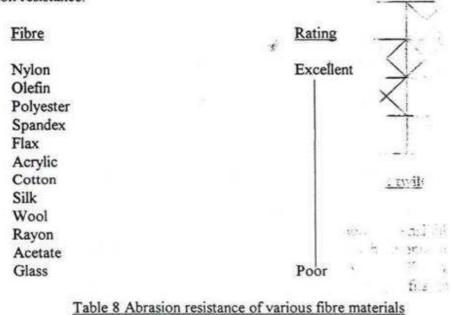
From Table 8, the abrasion resistance of various fibre materials5 was shown. It is observed that wool has a very poor abrasion resistance when compared with other raw materials (nylon, polyester, flax). Besides, as the Dref-yarn produced is consisted of a high percentage of short fibres, the above two factors result in a low abrasion resistance of the fabric produced.
